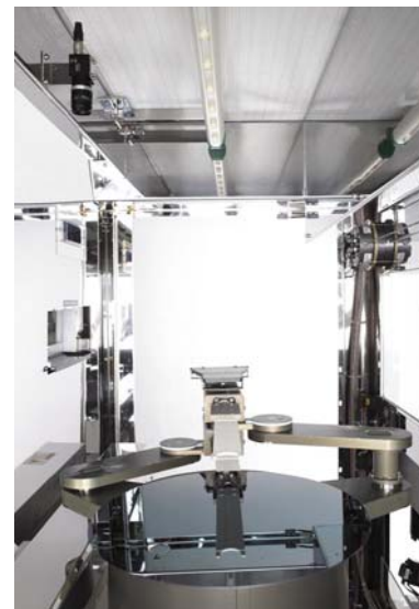
A Class 1 Mini-environment with fully sealed SCARA Robotics.
